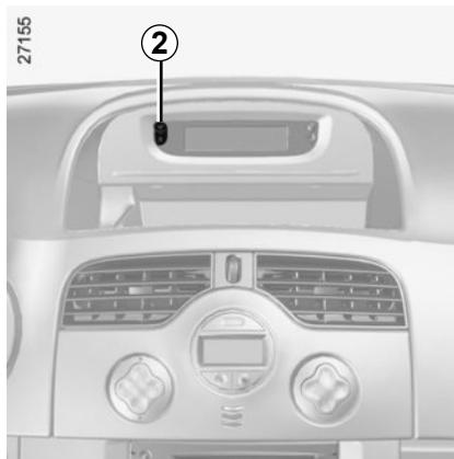
With the ignition on, you must check that the
