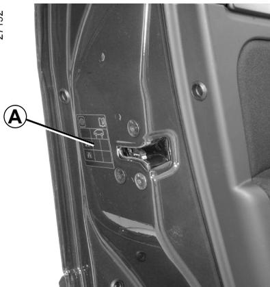
The tyre pressure is indicated on label **A** affixed to the edge of the driver's door. Open the door to read it.
