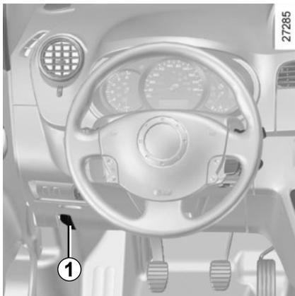
To open, pull handle **1**, located on the left-hand side of the dashboard.
