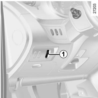
Control knob **1** is used to adjust the height of the headlight beams according to the load.
