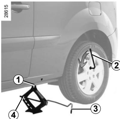
Use the wheelbrace to slacken off the wheel bolts **2**. Fit it so that you press downwards rather than pulling upwards.
